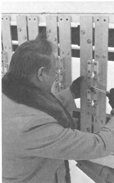
Figure 15. Bolting the specimens to the strain cycling weathering rack
