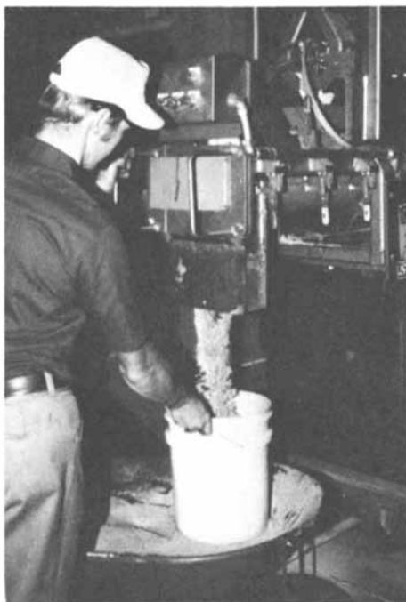
Figure 1. Continuous foundry mixer
